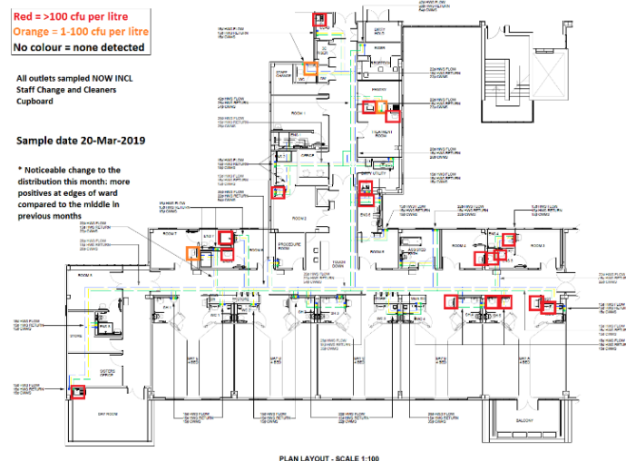
Figure 1 - West Bergholt pattern after multiple rounds of remedial actions (Mar 2019)
